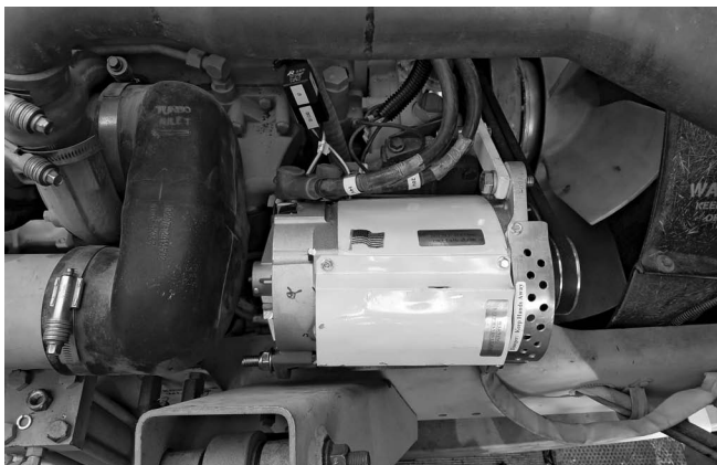
Double-Alternator mounted on a Cat engine as used in the MTV, LMTV, M1078, and many M-Series vehicles.
